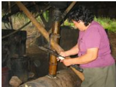
Repairing an alcohol distillation tank with banana pulp
